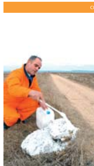
Marking parcels of land prior to aerial digital photography, Zadar county
