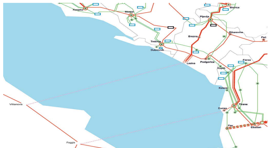
Existing and planned transmission corridors in Montenegro.
